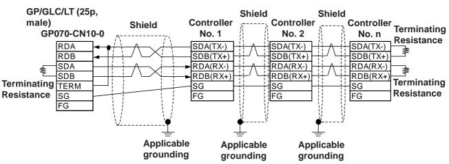
Cable Diagram 2 (1:n) (RS-422 4 Wires)
